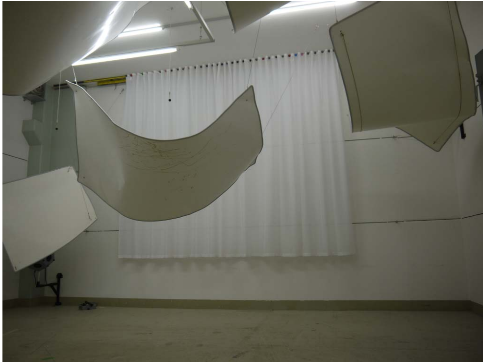
Figure B.1. Test object mounted in the reverberation room
