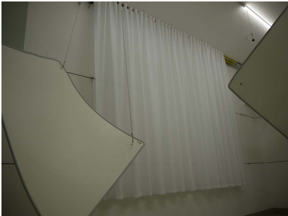
Figure B.2. Test object mounted in the reverberation room
